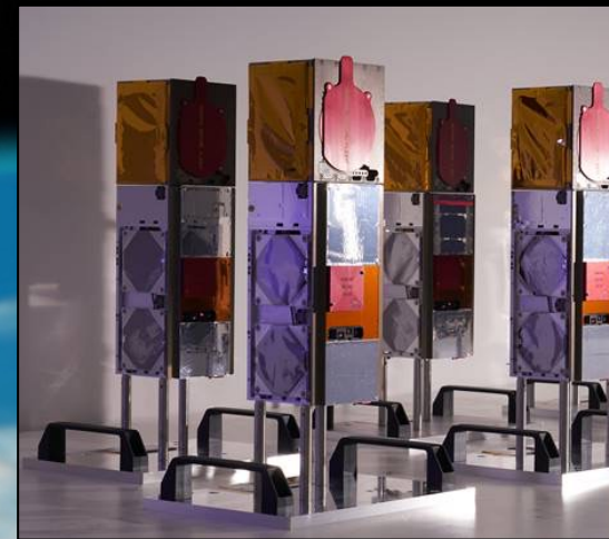
Constellation of Four 3U CubeSats MIT LL payload; BCT bus; KSAT downlink
